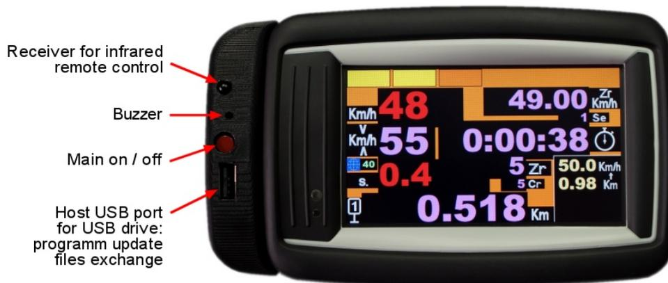
**Important:** the plastic case manufactured by 3D printing **does not withstand the temperature that can be found in a closed car, under a windshield, in the summer sun.** Therefore, if your car must stay parked in the sun, we advise you:
