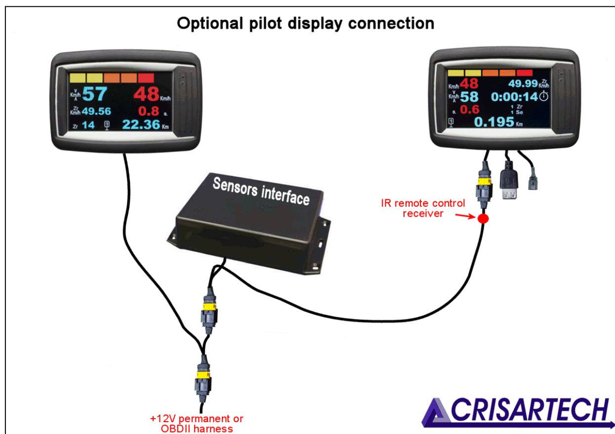
**Caution:** the infrared receiver for remote control is placed on the harness, just below the display connector. It must be ensured that lens is not masked and turned towards the co-pilot so that the infrared remote control is fully operational.
