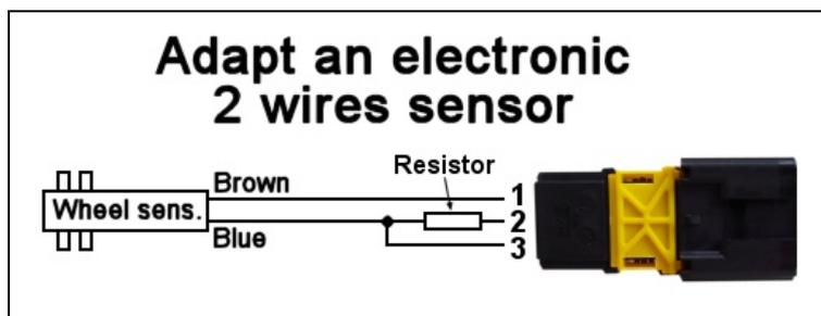
The resistance to put between the blue wire and the mass is 750 Ohms 1/4 watt for the sensors:
