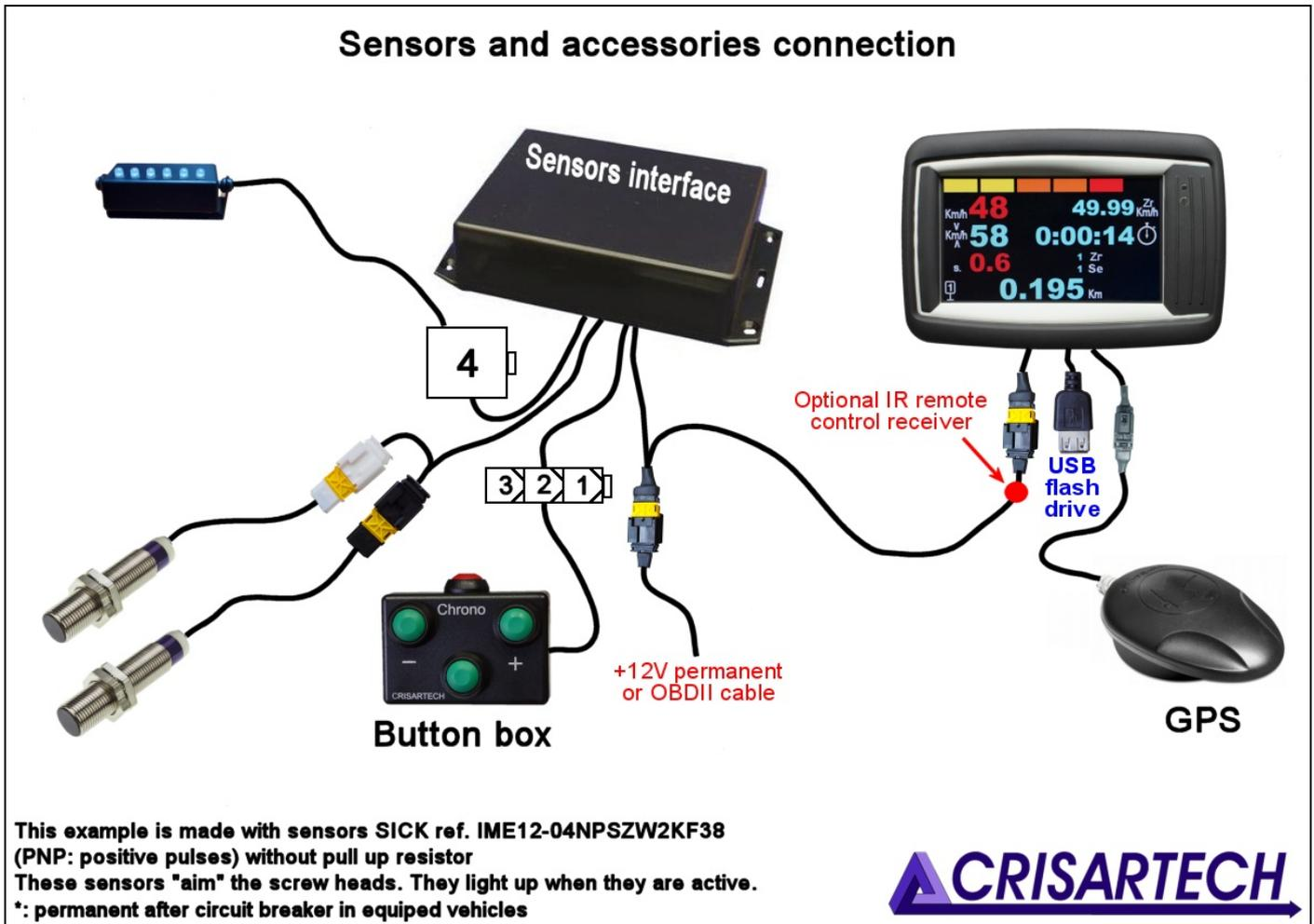
**Warning:** the interface provides a power supply for the sensors which is protected by a fuse. A fuse holder is located on the side of the housing. A 200 mA fuse is supplied as standard (plus a replacement fuse). This value is suitable for most sensors on the market, but it is up to the installer to check if it is correct for sensors other than those supplied by CRISARTECH.
