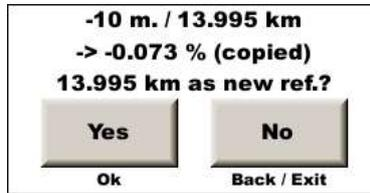
He therefore has a clear idea of the necessary calibration adjustment, in meters / km and in percentage. **The percentage is memorized by the device for use in the fine-tuning calibration page** (see below). The distance reference is the starting point for the cumulative correction, usually reset to 0 at the start of a RT. The percentage calculation is made from this point, up to the distance where the co-pilot pressed the **Info** button on the remote control. The co-pilot then has two options:
