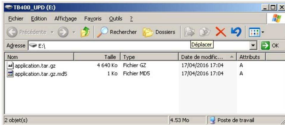
Insert the USB drive into the connector, the dash read it. In the screen automatically opened, a button appears if **both files are found at the "root" of the drive:**
