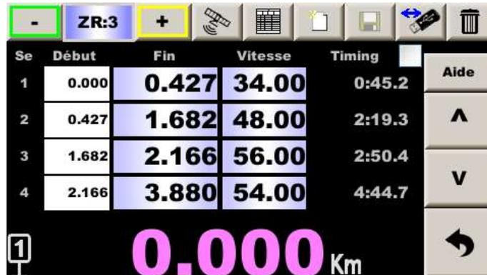
For each speed segment (**Se**, left column), enter the end distance and the average speed. The corresponding timing is displayed progressively in the right column, which allows to control the accuracy with some road-books that give these indicative values.
